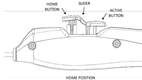
In Home Position the Slider is retracted, and the distal mechanism is drawn into the Distal End.
