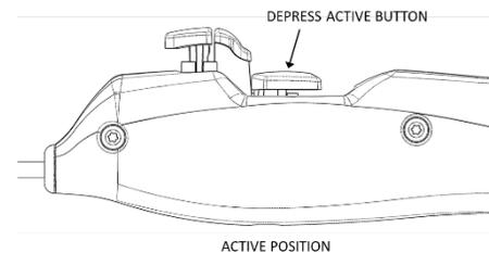
With the device in Open Position, the Active Button is pressed and held to expose the Blade. The hook shape is maintained while the Active Button is depressed. By releasing the Active Button, the device is returned to Open Position.
