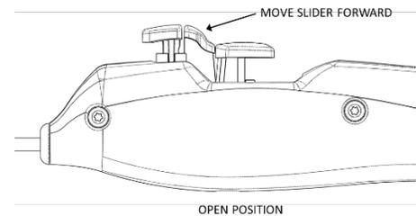
The Slider is moved forward to deploy the Hook into Open Position. When the Slider is fully forward the Hook will lock into position until the Home Button is depressed to return to Home Position.
